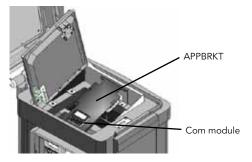
Reapply controller power and verify that the Com module display lights up and displays characters.
