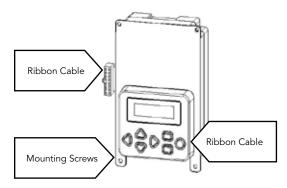
The ACC-COM-LAN provides Ethernet communications for ACC/ AGC series controllers from a central computer.
