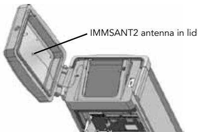
Open the facepack frame in the top of the pedestal, to expose the communications module mounting area.
