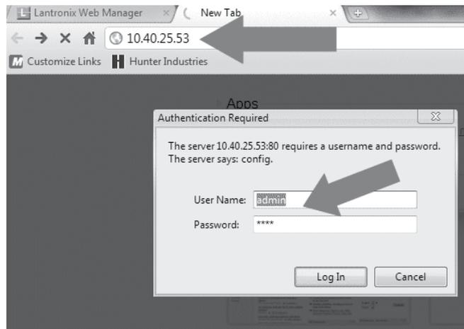
Use a computer on the network (usually the central control computer) and enter the initial IP number of the Com module in the address line of any internet browser.
