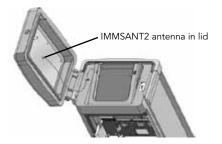
Open the facepack frame in the top of the pedestal, to expose the communications module mounting area.
