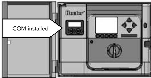
The ACC-COM-LAN may also communicate with other controllers, via optional UHF radio modules (sold separately) with an antenna for wireless communications, and/or an ACC-HWIM hardware interface module (sold separately) for hardwired communications over Hunter GCBL cable. The other controllers will not have an IP address, and will use the controller address only for hardwire and radio communications.
