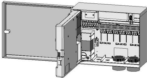
2. Remove the facepack door frame: Disconnect facepack door frame ribbon cable, open and lift up the door frame to compress the top hinge, and tilt out of the lower hinge.
