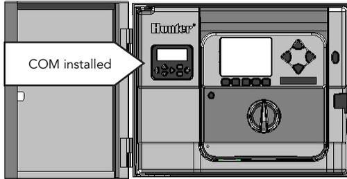
The ACC-COM-GPRS is another version of the module which includes a Site Plan, meaning it can link to other controllers on a site with hardwire or UHF radio communications. This requires a Hunter Site Plan account.
