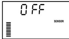
**SENSOR BYPASS** position to disable the rain sensor from the system to allow for the controller operation. You can also bypass the weather sensor for manual operation by using the **MANUAL - SINGLE STATION** function.
