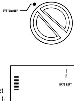
4. Turn the dial back to the **RUN** position at which time, **OFF**, a **number** and the **DAYS** icon all remain on.
