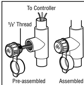
3. Screw the SmartPort harness housing into the "Tee" as shown.
